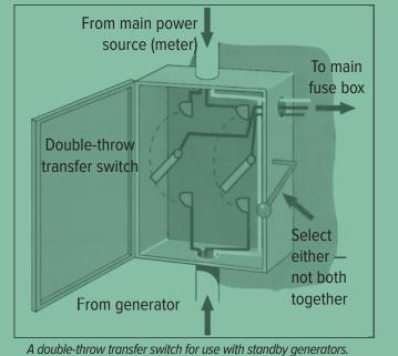
A double-throw transfer switch for use with standby generators. Consult a licensed electrician to install a switch like this if you use a standby generator — it's the law!
